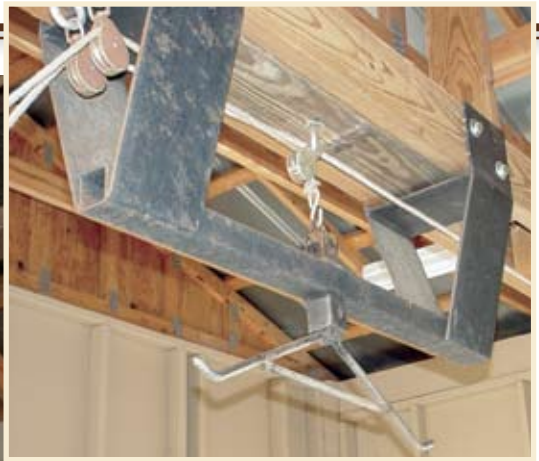
These two gambrel systems are homemade designs, described in the article, that prevent the gambrel from spinning.
