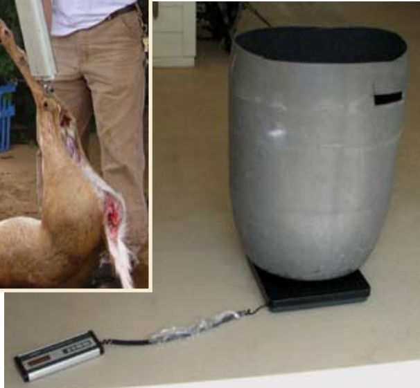
Dressed body weights are critical data. When using a spring scale (left) to collect weights, use an object with a known weight to regularly check the scale's zero calibration. A digital platform scale like the one below is more expensive but much more accurate.
